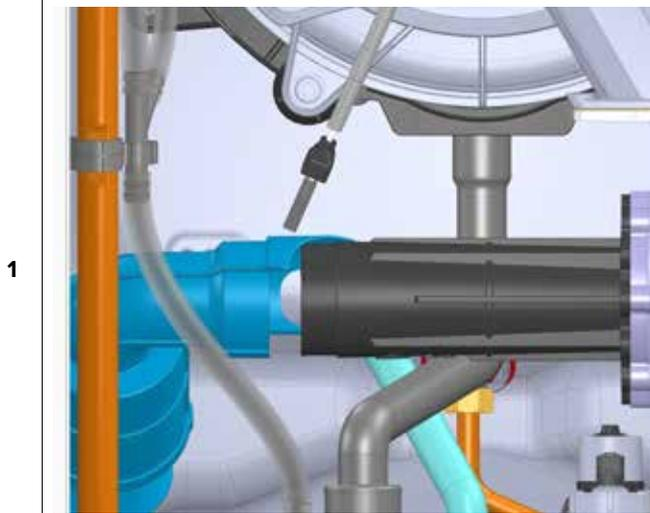
Remove the two screws and remove the heat exchanger
