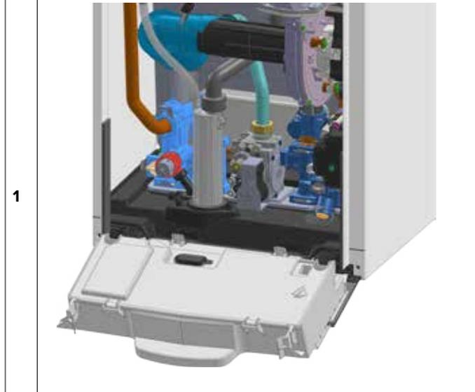
Unhook the two clip and remove the cover
