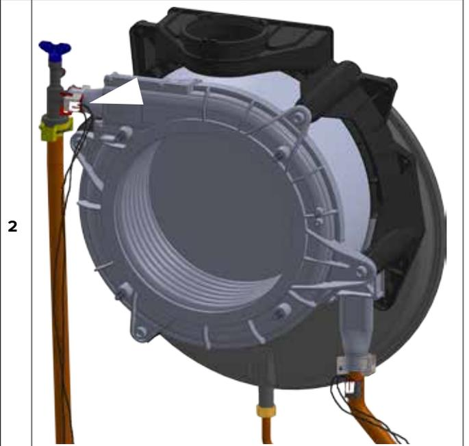
Remove the clip and the temperature sensor
