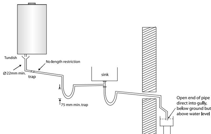
4. External termination of condensate drainage pipe via condensate siphon
