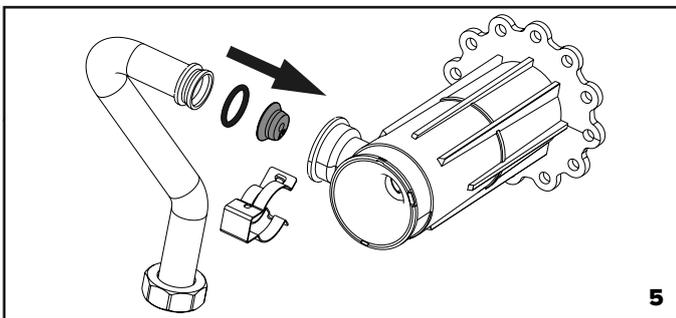
7. Reassemble the gas supply onto the venture assembly (fig 4) and reattach the silencer.
