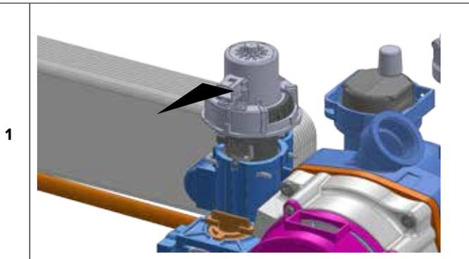
Rotate clockwise to unhook the locking ring.
