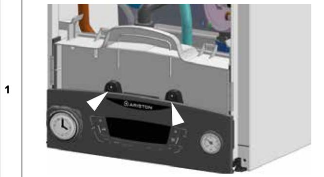
Disconnect the electrical plug connections.
