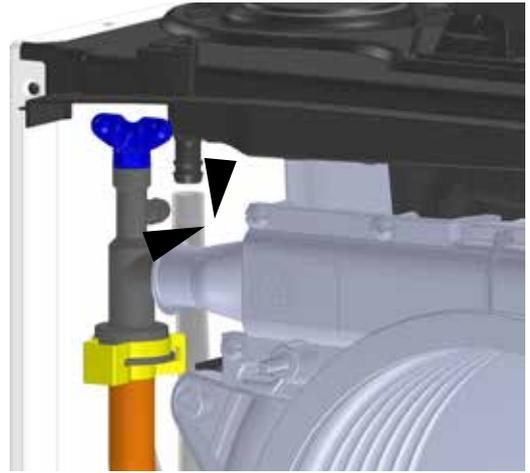
Disconnect the heating flow pipe
