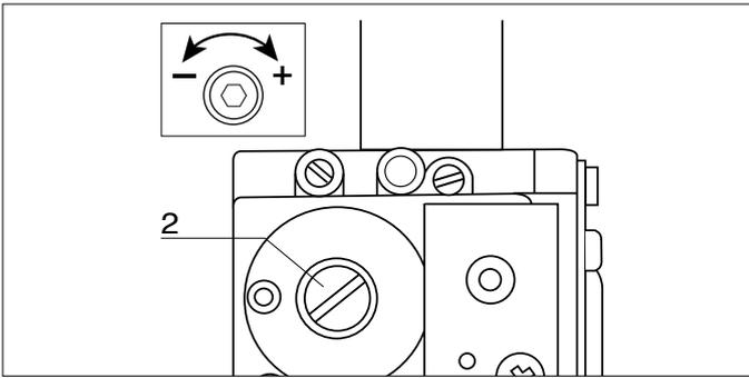
If the value measured corresponds to the value given in the table, adjustment is complete, otherwise start the setting procedure again.
