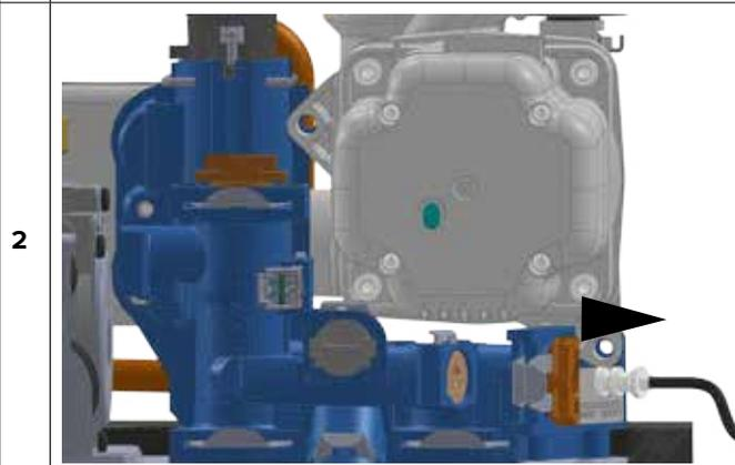
Remove the clip and remove the filter
