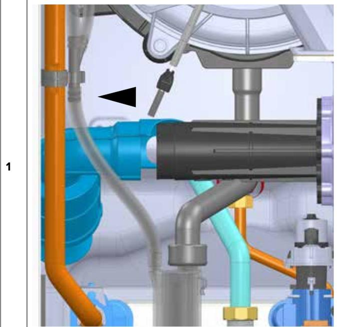
Isolate the gas supply and disconnect the gas pipe.
