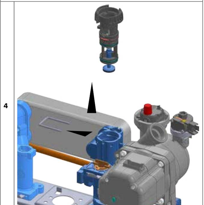
**WHEN REASSEMBLING, ENSURE THE DIVERTER VALVE IS ALIGNED CORRECTLY.**
