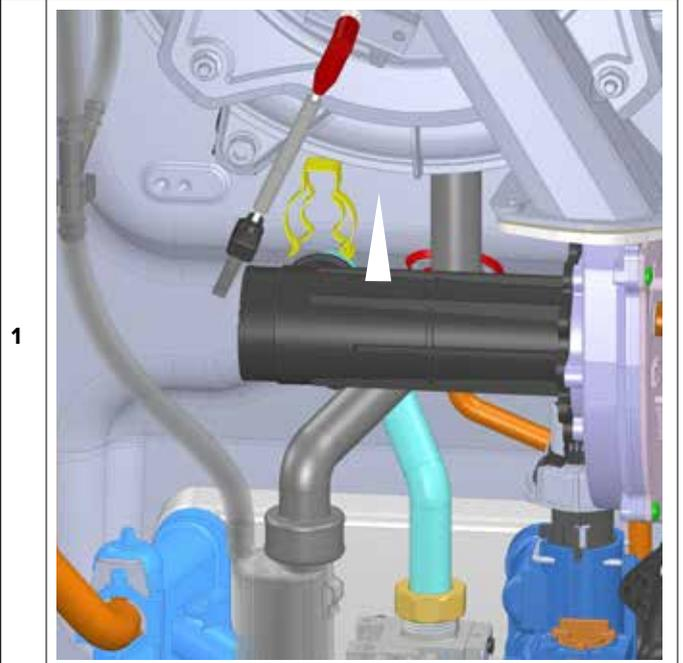
Remove the three screws to free the fan.
