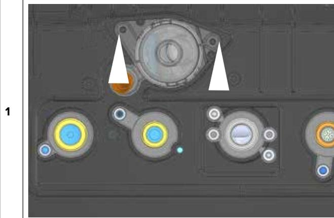
Disconnect the condensate pipe from the condensate trap
