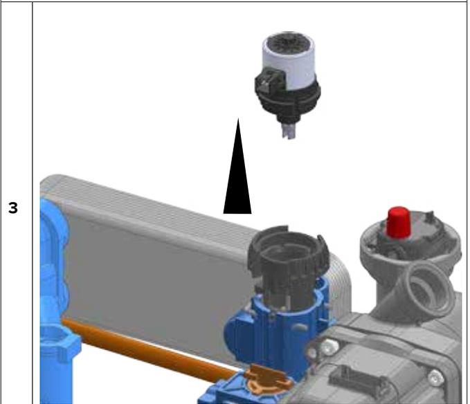
Remove the clip and lift the diverter valve from the assembly.
