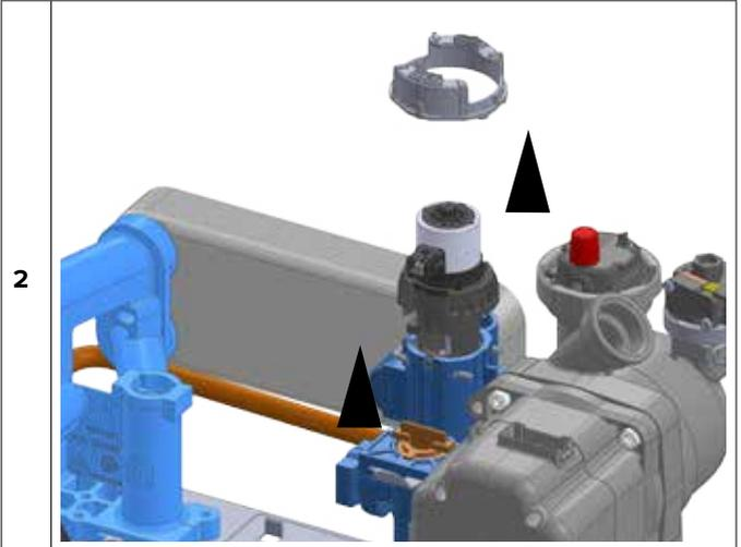
Remove the 3 way valve motor.
