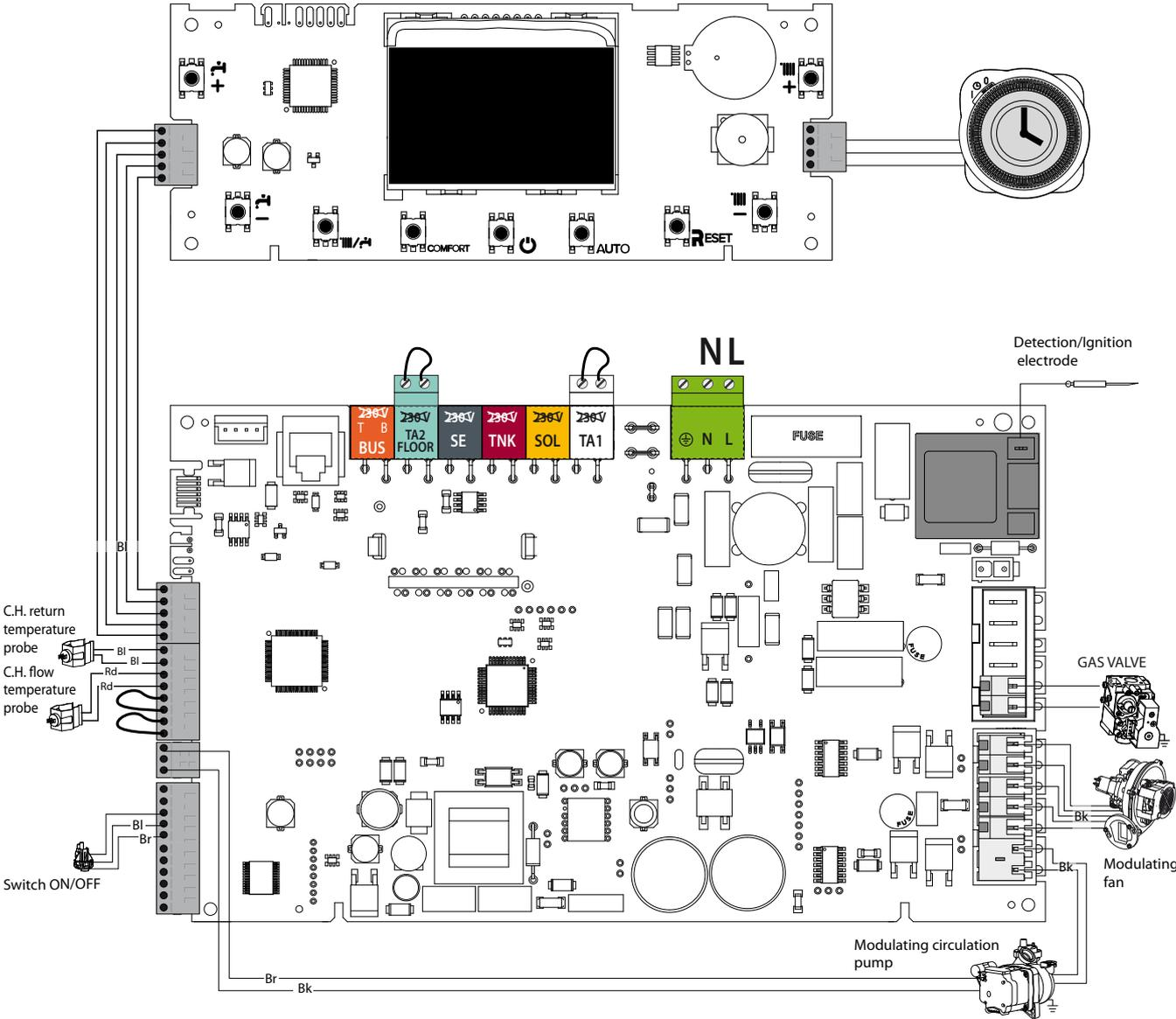
S plan wiring diagram.
