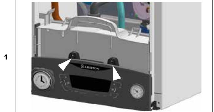
Disconnect the electrical plug connections and unhook and remove the P.C.B.
