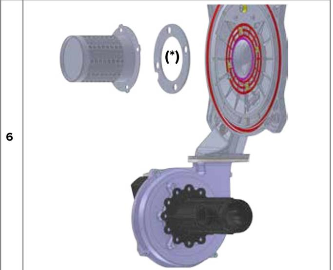
**Verify and replace the other gaskets** if they are damaged or showing signs of deterioration
