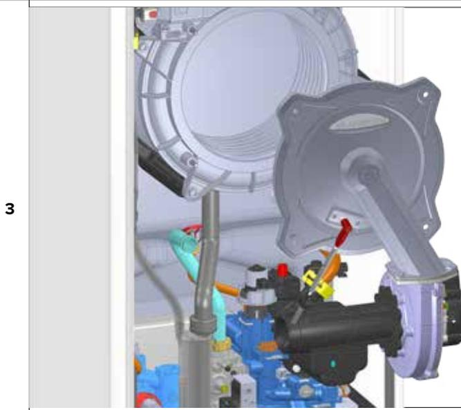
Remove the two screws and remove the electrode
