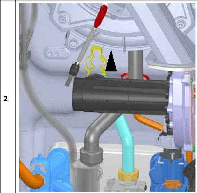
Disconnect the cable of the electrode.
