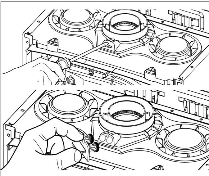
**Operation 3 - Adjusting the CO2 at maximum gas flow rate (domestic hot water)**
