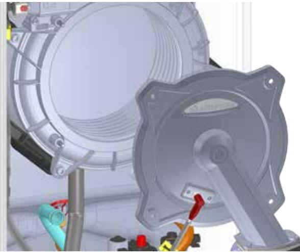
Remove the two clips to disconnect the exchanger on the heating flow side
