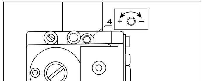
If the value measured corresponds to the value given in the table, max adjustment is complete, otherwise start the setting procedure again.
