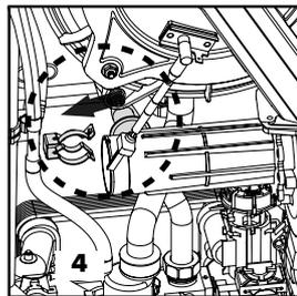
5. Disconnect the gas supply from the venturi assembly (fig 4)
