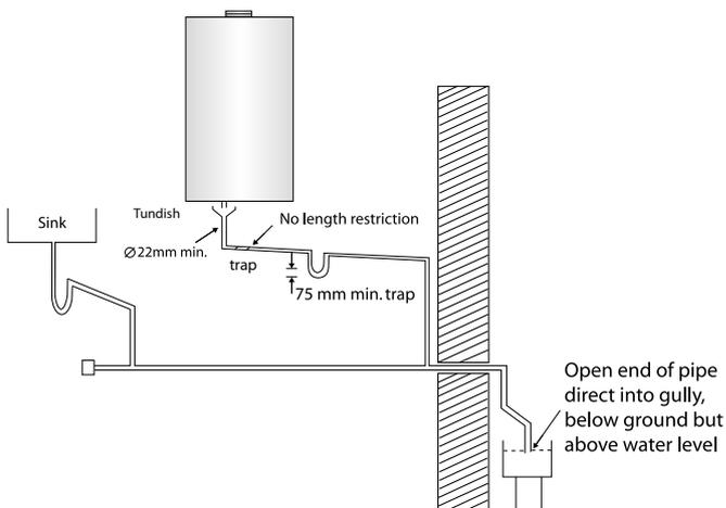
3. External termination of condensate drainage pipe via internal discharge branch (e.g. sink waste - proprietary fitting).
