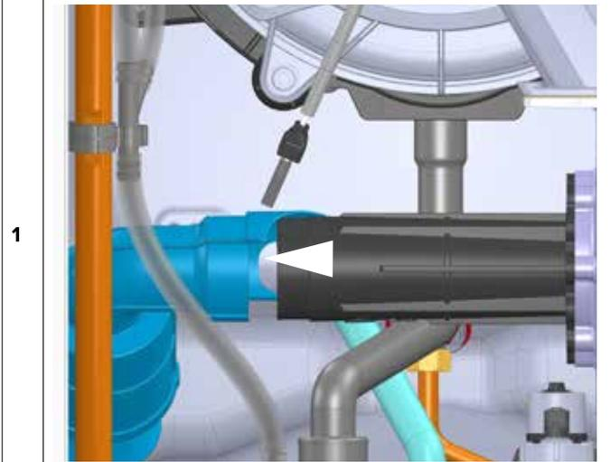
Isolate the gas supply. Disconnect the gas pipe.
