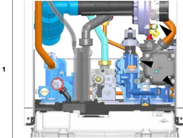
Disconnect the pipe and then move the pump to the right to disengage
